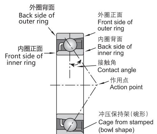
Double-row angular contact ball bearing has such two types of structure as one outer ring and two inner rings and one outer ring and one inner ring.
